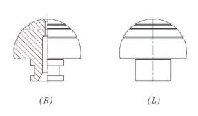
IT IS DIFFERENT SHAPE BETWEEN R TYPE AND L TYPE OF BALL
