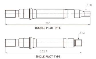
IT IS DIFFERENT SHAPE BETWEEN DOUBLE AND SINGLE PILOT TYPE OF DRIVE SHAFT
