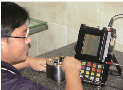
Inspection for Brass Brazing with Ultrasonic Test
