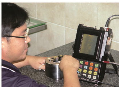
Inspection for Brass Brazing with Ultrasonic Test
